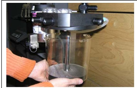
Fill in the soda lime into the canister. The filling sign gives you the max. quantity, do not exceed this line. Plug on the canister and move the closing mechanism to close it. Please take care that no soda lime is in the centre-tube.
